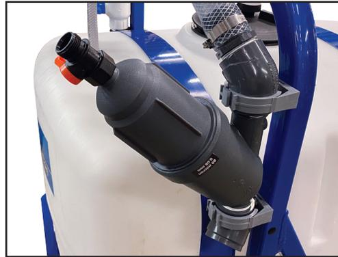
The FCST100 includes a check valve to prevent water hammer from damaging the injector. This must be used to maintain the injector warranty.
